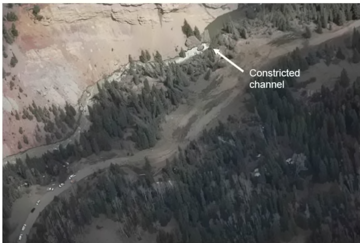
Figure 4-26 Constriction of the San Juan River by the Toe of the East Fork Landslide
